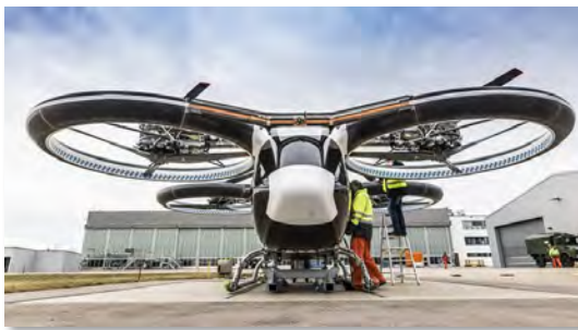
City Airbus, four-seat multicopter vehicle demonstrator
