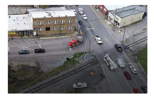
At the South intersection, a truck turning right from U.S. Highway 31 southbound onto State Route 25 encroaches slightly into the eastbound through lane on State Route 25.
