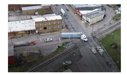
Furthermore, at the North intersection, a truck turning right from U.S. Highway 31 northbound onto State Route 25 encroaches significantly into the westbound through lane on State Route 25. An example of this encroachment at the north intersection is shown in the following photograph.
